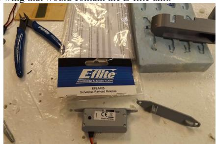
The first units printed had an open side so we could see how much space would be needed for the wire and connector. We got the size correct on the first attempt. I simply glued a piece of styrene over the open side, mission complete.
