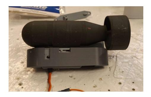
I made a RTV mold to produce multiple copies of the part that attaches to the bomb to the release. If anybody is interested Jim will print up the mounts for \$6.00. If anybody wants to print their own Jim will email them the G Code. Each release comes with one part that attaches to the bomb. I can make additional parts for .40 cents.
