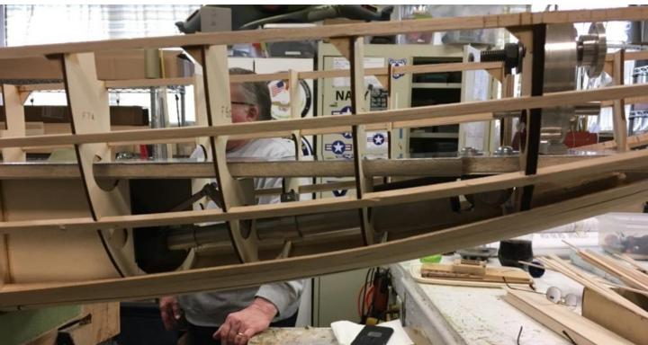
A few days later we hit a small snag. While lining up the Torque Plate noticed a small deflection in the Propeller Shaft. It is possible the nose bearing holder would prevent a small wobble this from becoming a problem. We developed a couple of other solutions,
