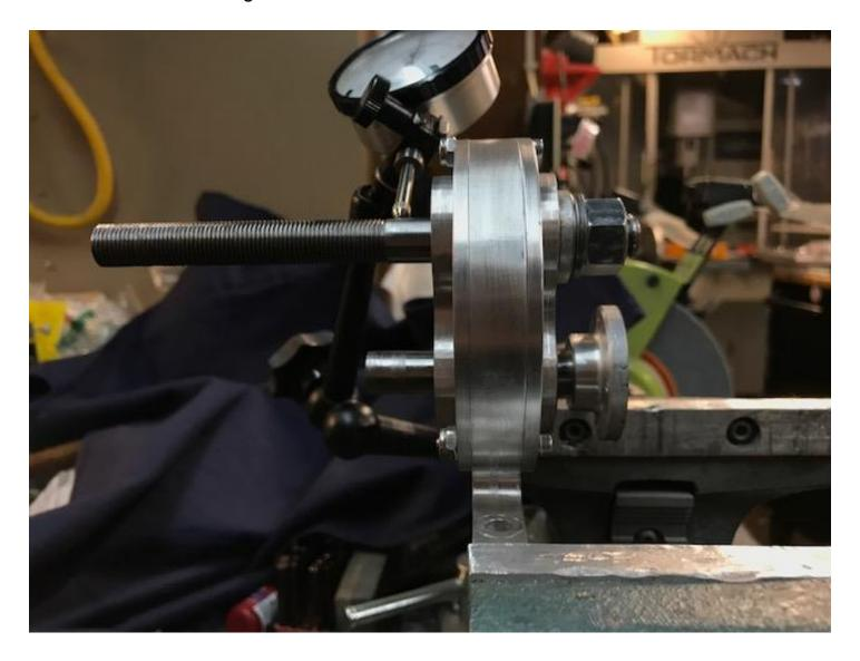
The new shaft has been run up over 2000 rpm with no deflection.
