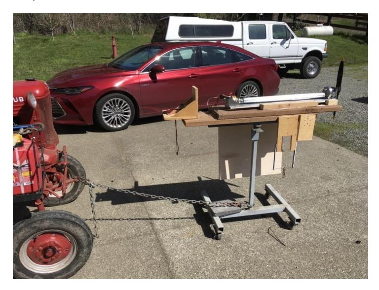
We never got past half throttle because we had one of the driveshaft tube screws kept coming loose. After about three minutes it would back out about half way. We couldn't tell if the Locktite failed, or did we forget to apply it. We don't know. We decided let's just go ahead and safety wire all the screws on the rotating parts and get on with the testing. We also decided to add a hard point below the ESC on the motor mount to allow us the attach the strain gauge to the motor centerline.
