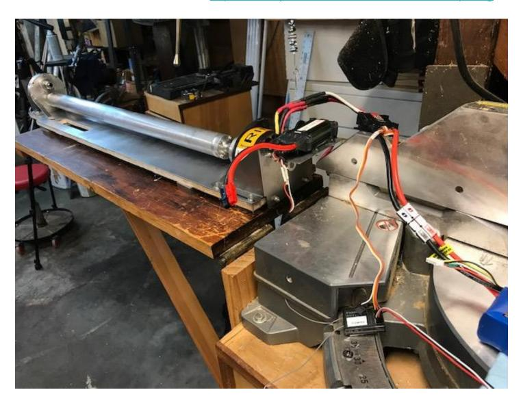
The first run was conducted using a 4s battery. Things went smoothly although the thrust bearing retainer nut on the gearbox loosened. We did notice a slight amount of wobble on the shaft coupling on the motor end. The drive tube is bonded to the shaft coupler we may have relook at that. Next, we will secure the Torque Plate to a test fixture and run it
