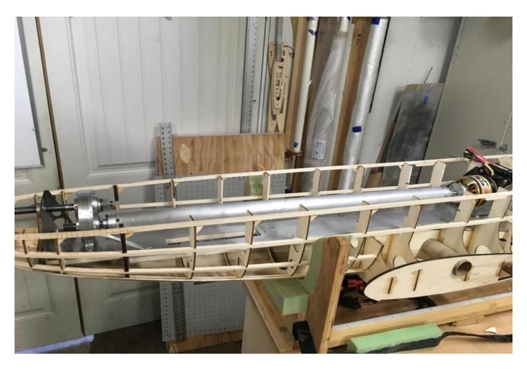
Next, we clamped the unit on the bench and ran it for a while on 6s. We recorded the watts and amps at 25% and 50% throttle. Everything seems fine so lets put a propeller on and do some low speed running.
