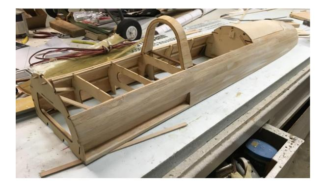
fuselage is no longer flat. I can slide a 3/32 piece of balsa under. When planked it was done on both sides at the same time and it remained flat on the bench. Apparently, the balsa sealer caused the shrinkage. I will hose the inside down with denatured alcohol and firmly weight it down, till it dries flat. Two steps forward......
