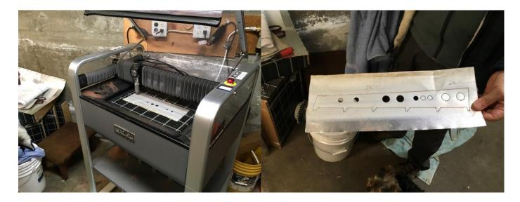
We verify our cut on the plans and something is very wrong. The gussets to increase the surface contact area to the flap ribs are mostly too small and some are incorrectly spaced.
