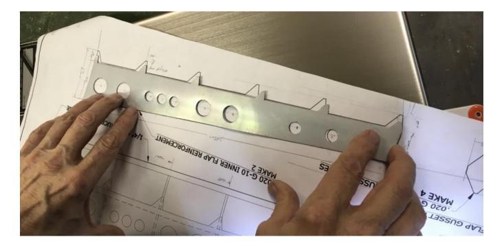
The shape and size are ok. The outline has all the correct angles. Surely it is something caused by having to convert the basic drawing through two additional programs till the cutter understands what we want. We will get there, but for now we are stuck. Later: Jim got it figured out, corrected and made a test cut on the thicker .032 not the .016 we intend to use. Then this happened, the G-10 delaminated.
