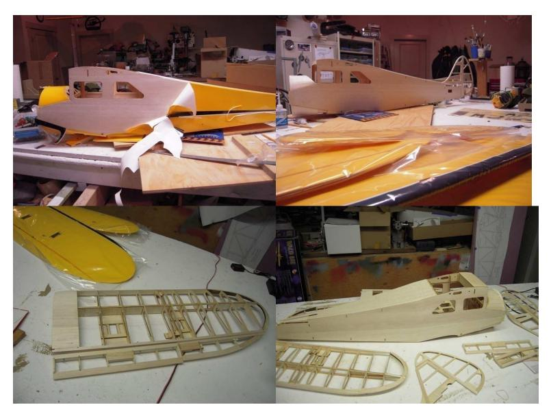
After the covering was removed I re glued every joint I could get to. Since the plane was going to be electric I had to build a new motor mount and batteries rack. I also beefed up the landing gear mounting base.
