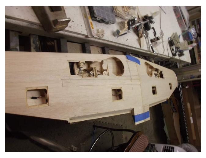
When the epoxy had dried I sanded the bottom of the wing and applied a Carbon Fiber strip to the skin over the spar. Two coats of West System Epoxy was used to bond the Carbon Fiber.
