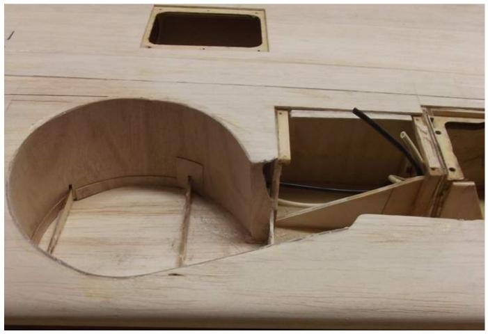
That takes care of the right wing. The the air lines and servo extensions have been installed.
