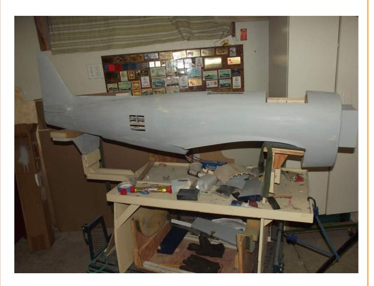
Two heavy coats of primer were applied to fill the cloth weave. Most of which will be sanded away to a smooth finish.
