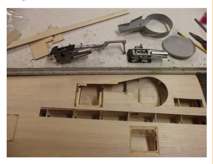
The wing uses an aluminum joiner sandwiched between two light ply outer skins that slide about eight inches into the wing spar box on both sides of centerline. I think I will reinforce from centerline out one rib past the landing gear bay.
