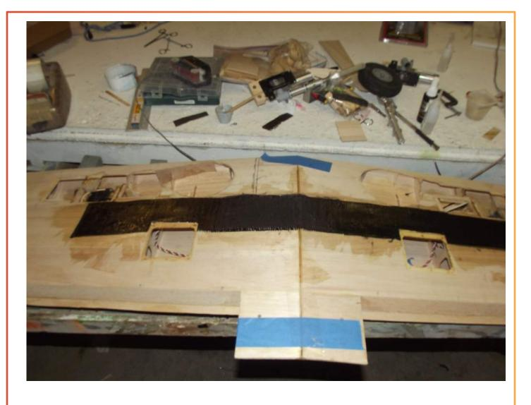
Once the Carbon Fiber is sanded and smoothed into the wing I will cover the wing with ¾ ounce fiber glass cloth. The shape of the wing is such the flat landing gear doors that came in the kit won't contour to the wing shape so it will be necessary to lay up fiber glass main and secondary gear doors.
