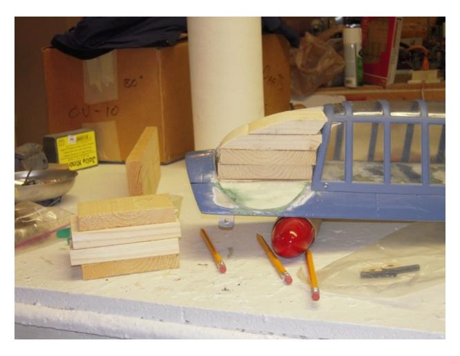
First the turret area was decked over and filled in. Then a series of pine boards were rough cut to the basic canopy shape. A piece if 1/8 inch ply was accurately cut to shape to use as a sanding guide.
