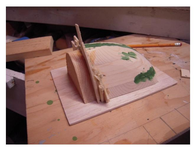
Additional wood is added to make the part oversize so there is excess plastic web to cut off.
