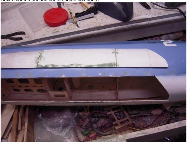
I removed some of the fuselage strength when I cut out the bottom, So I attached  $1/4 \times 3/8$  oak stringers just inside and above the door cut outs. These stringers run fro the firewall to about a foot behind the doors.
