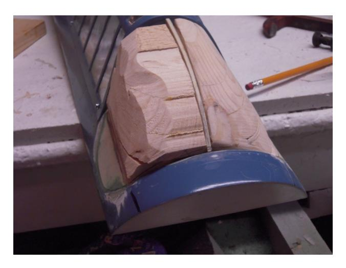
Now the rough sanding and grinding takes place. This is about an hour job on a good belt sander. In this process there is a bunch of sand and fit and sand and fit. You need to work slowly here. you can't unsand the wood back on. After the basic shape is completed you now need to prepare your piece as a mold master. Since we are doing to be vaccuforming in clear plastic the mold has to be as smooth as possible.
