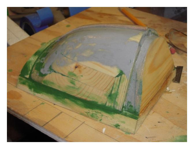
Notice how additional wood has been added on the front back and bottom of the master.
