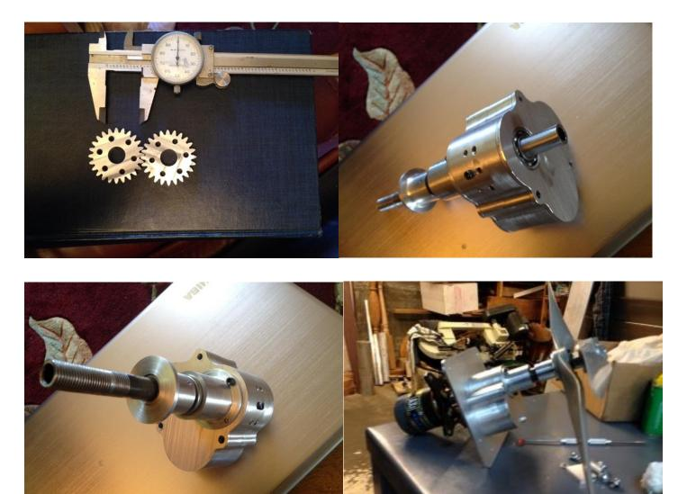
We decided to use an AXI 5345/16 for power. Ok now we need to test this monster. Earlier we had built a test stand to test motor and propeller combinations. We conducted many tests at progressively higher power settings. The first time we ran it, it started rolling down the driveway. We experienced a few problems had some bearing failures, loose gears that type of thing. We even had the propellers come in contact once.
