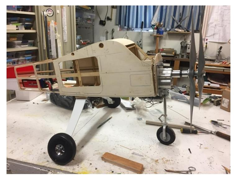
To change the angle of attack on the fuselage we ordered a new wider, taller and stronger aluminum main gear from TNT Landing Gear. The aircraft in now ready for flight test.
